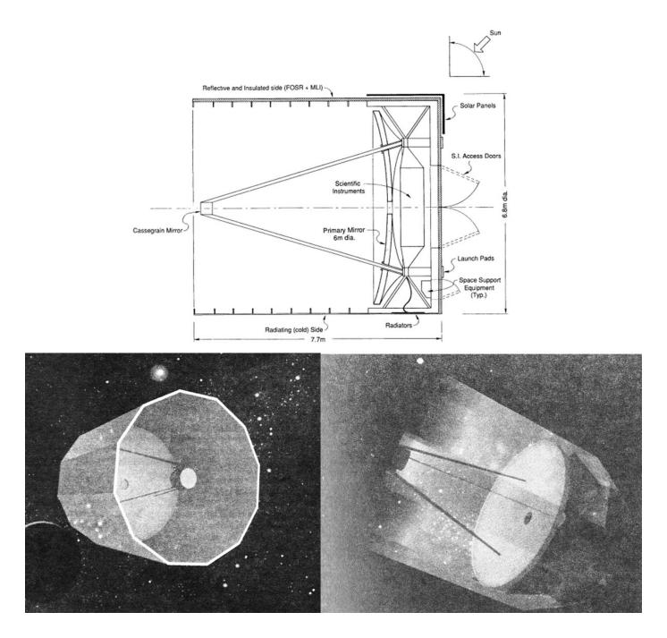
**Figure 2:** The *NGST* concept layout discussed by the UV-Optical in Space panel of the 1990 Decadal Survey, along with a couple of renditions. *JWST* looks very different from this early concept!
